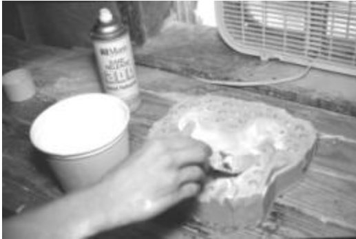
Aluminum trihydrate (ATH) is brushed onto the surface of the mold.
